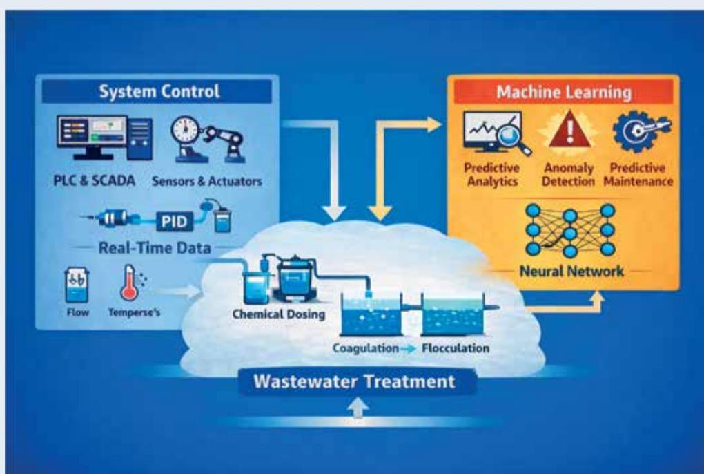
Fig 1. Schematic overview of a system control for coagulation and flocculation in wastewater treatment
